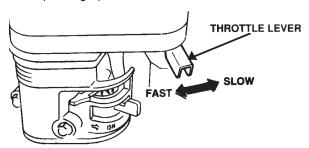
Figure 23. Throttle Lever
